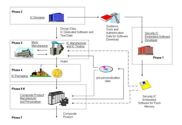
Figure 17: Security IC Life-Cycle if Security IC Embedded Software is loaded by Security IC Dedicated Software into the programmable non-volatile Memory
