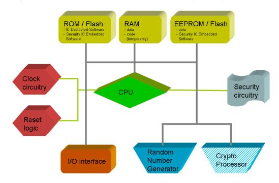
Figure 1: Typical Security IC
