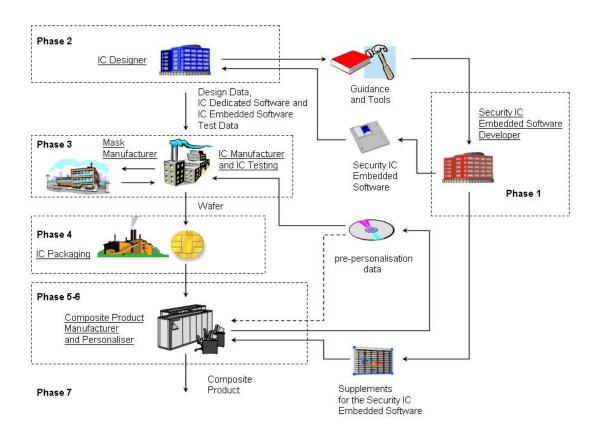
Figure 16: Security IC Life-Cycle if Security IC Embedded Software is implemented in ROM and EEPROM only
